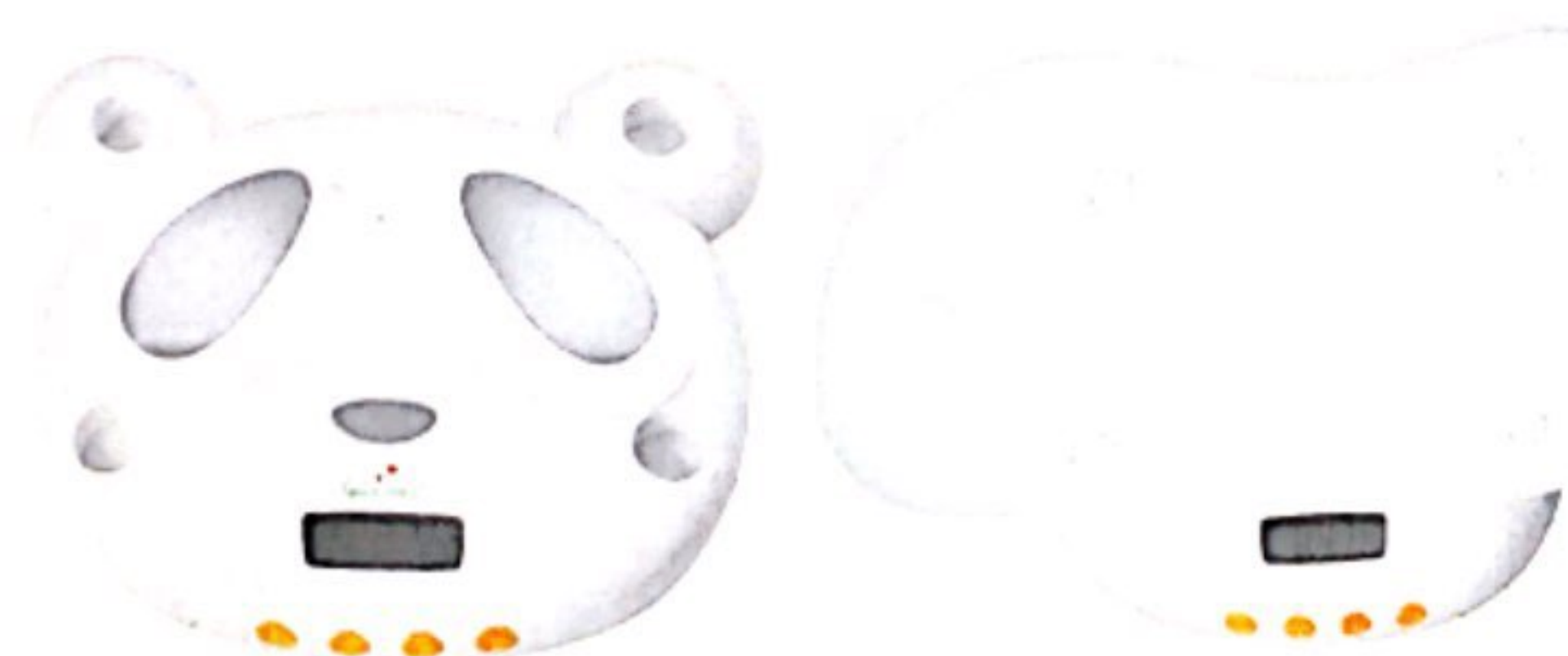
GT130-500 Baby Scale 1. Tray Size: 56X28X9.3cm Body Size: 36X29.5X7.5cm Net Size: 56X31.5X13.5cm 2. Max. weight : 30kg 3. Graduation: 5g 4. Lcd Display+auto Power Off +low Battery Indicator+1 Loadcell 5. Precision
