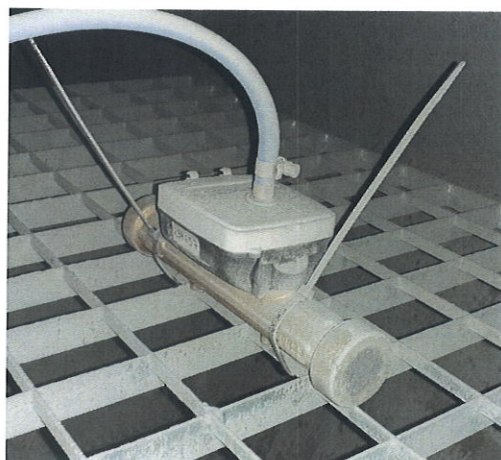
Specimen immediately after the end of IP6X test
