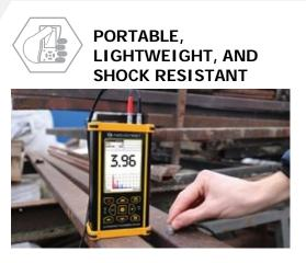
Ultrasonic thickness gauge UT-2A is a lightweight device that is useful in both difficult outdoor conditions and in workshops. The special rubberized housing will protect it against damage from drops.
