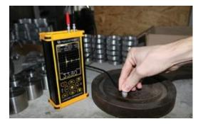
A-scan of the thickness gauge allows displaying the waveform of the signal for subsequent analysis. Viewing the reflected signals on the screen, users can eliminate false triggering and adjust the device as correctly and accurately as possible.
