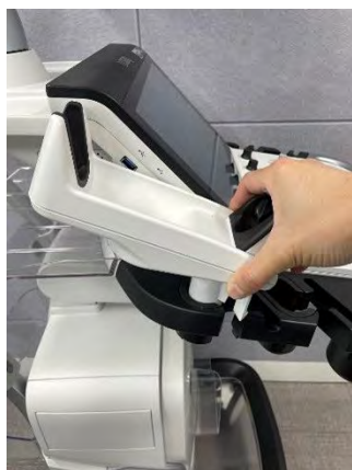
Figure 3-5 TVTR Probe Holder
