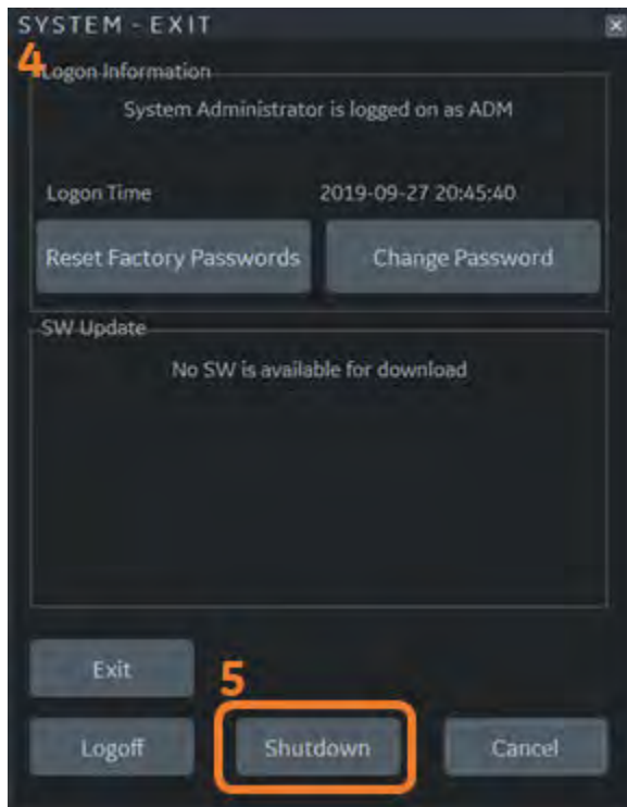
Figure 13-278 Shutdown to Begin Installation
