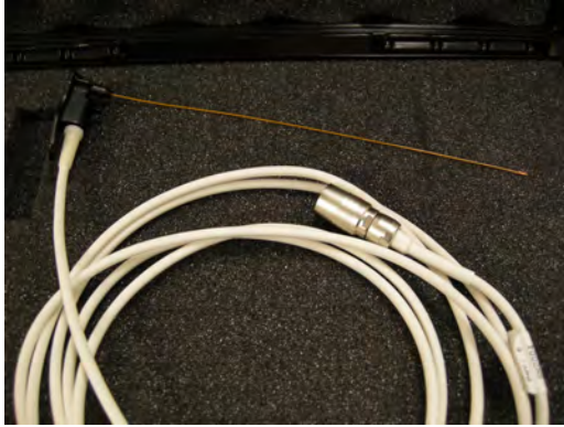
Figure 13-133 Needle Tip Sensor and Cable Close-up
