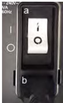
Figure 3-10 Circuit Breaker (a) and Power Plug (b)
