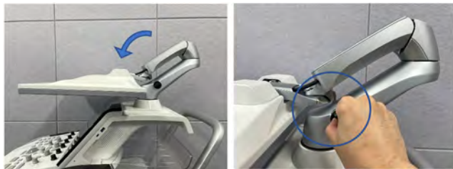
Figure 3-44 Flip down the monitor and lock the monitor arm
