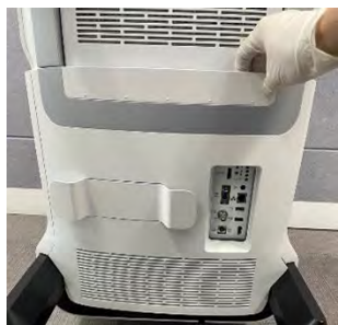
Figure 12-12 Remove the rear cover
