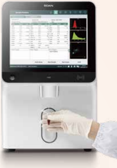
16 microliter of sample aspiration
