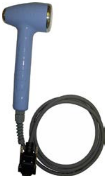
Figure 5. Ultrasound transducer with ERA of 7 cm 2 and 3 cm 2 .
