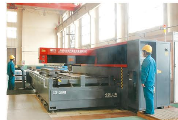
SLCF-*15*30B大型激光切割机 SLCF-*15*30B Giant Laser Cutting Machine
