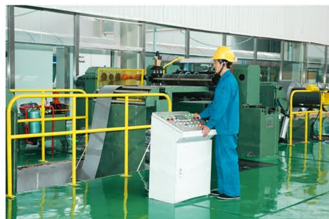
XBJI-05/05型硅钢带纵剪生产线 XBJI-05/05 type of steel slitting produceline
