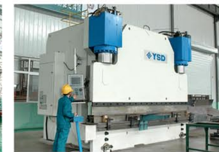
数控板料折弯机 CNC Bending Machine for panel veneer
