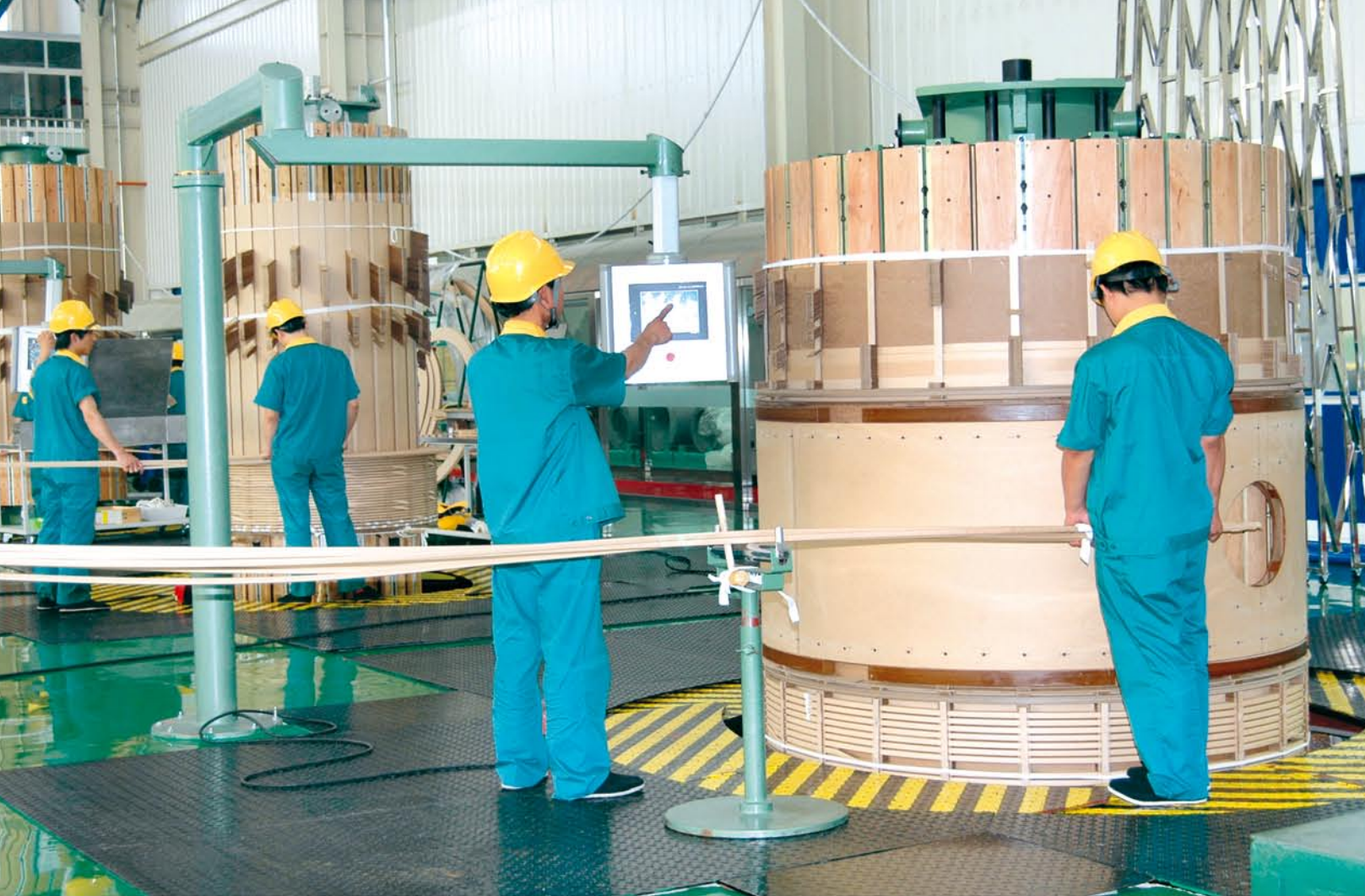
BR2-35/35大型立式绕线机 BR2-25/35 large vertkal winding machine
