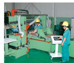
数控垫块机 Auto Cushion Marking Machine
