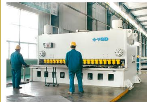
数控液压剪板机 CNC Cutty machine
