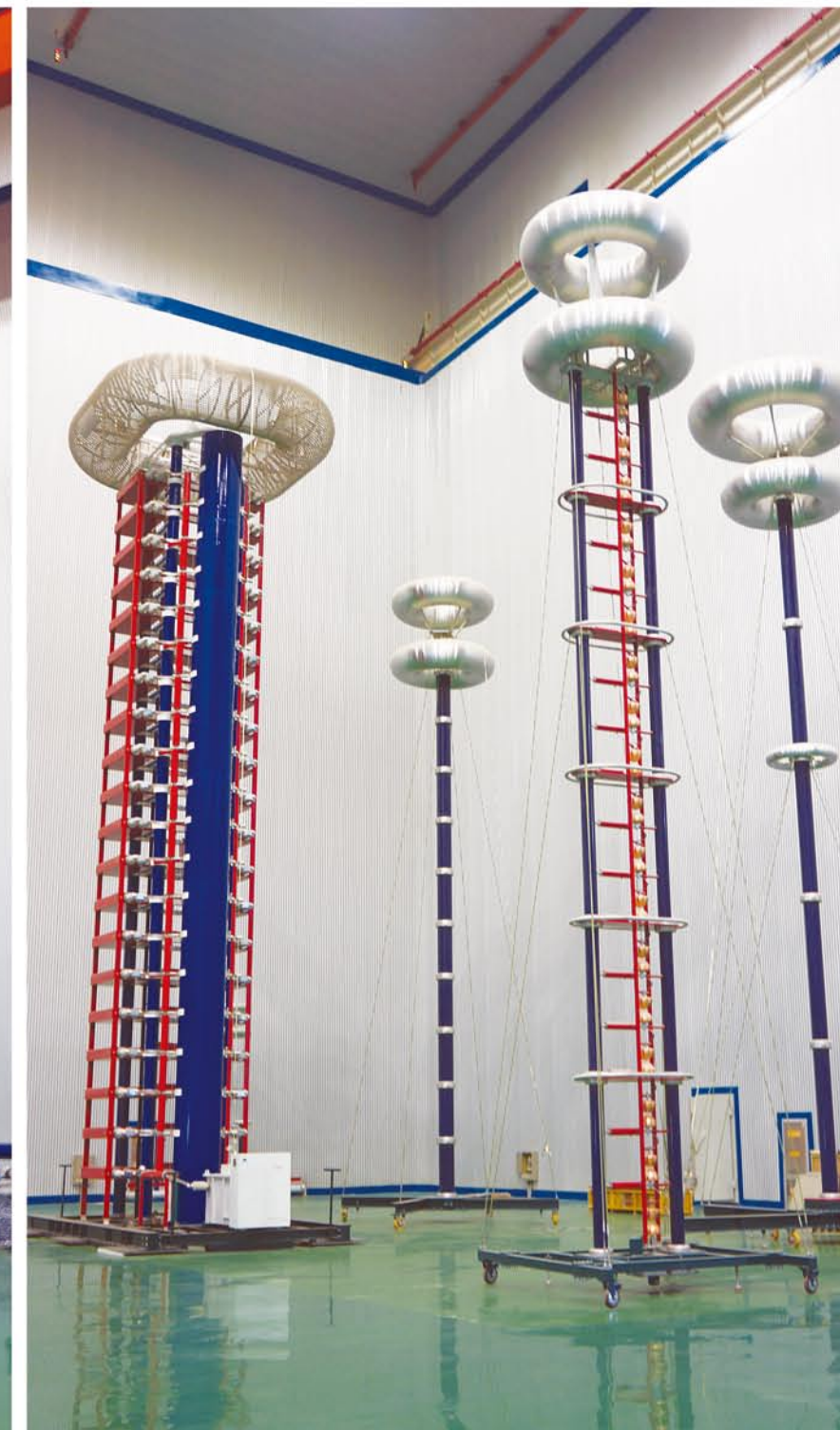
换流变试验大厅 converter transformers testing hall
