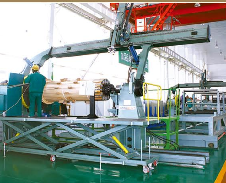
大型卧式绕线机 Large-Scale Horizontal Winding Machine
