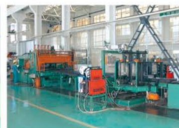
波纹油箱生产线 Corrugated Oil Tank Production Line
