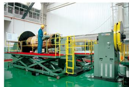
BR42-28大型卧式绕线机 BR42-28 Good-sized Horontal Winding Machine
