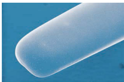
REM image atraumatic tip of a YASARGIL Clip from Aesculap; smooth surface prevents damage to tissue.
