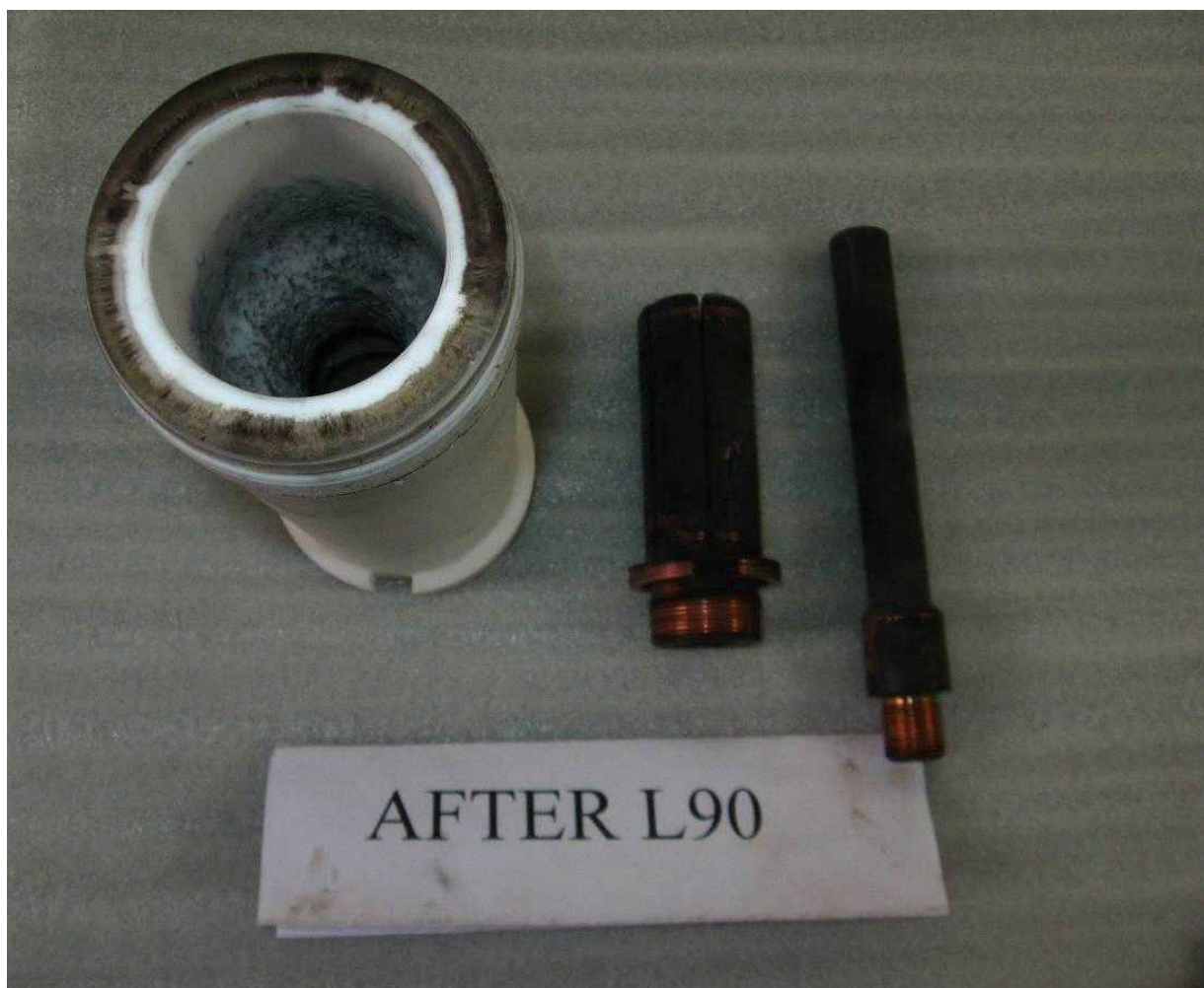
Photo. HP07 : Contact after short line fault (L90)
