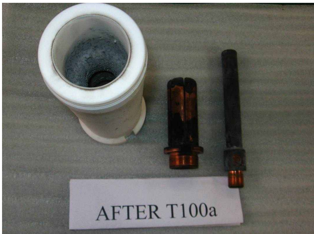
Photo. HP05 : Contact after basic short circuit test(T100a)
