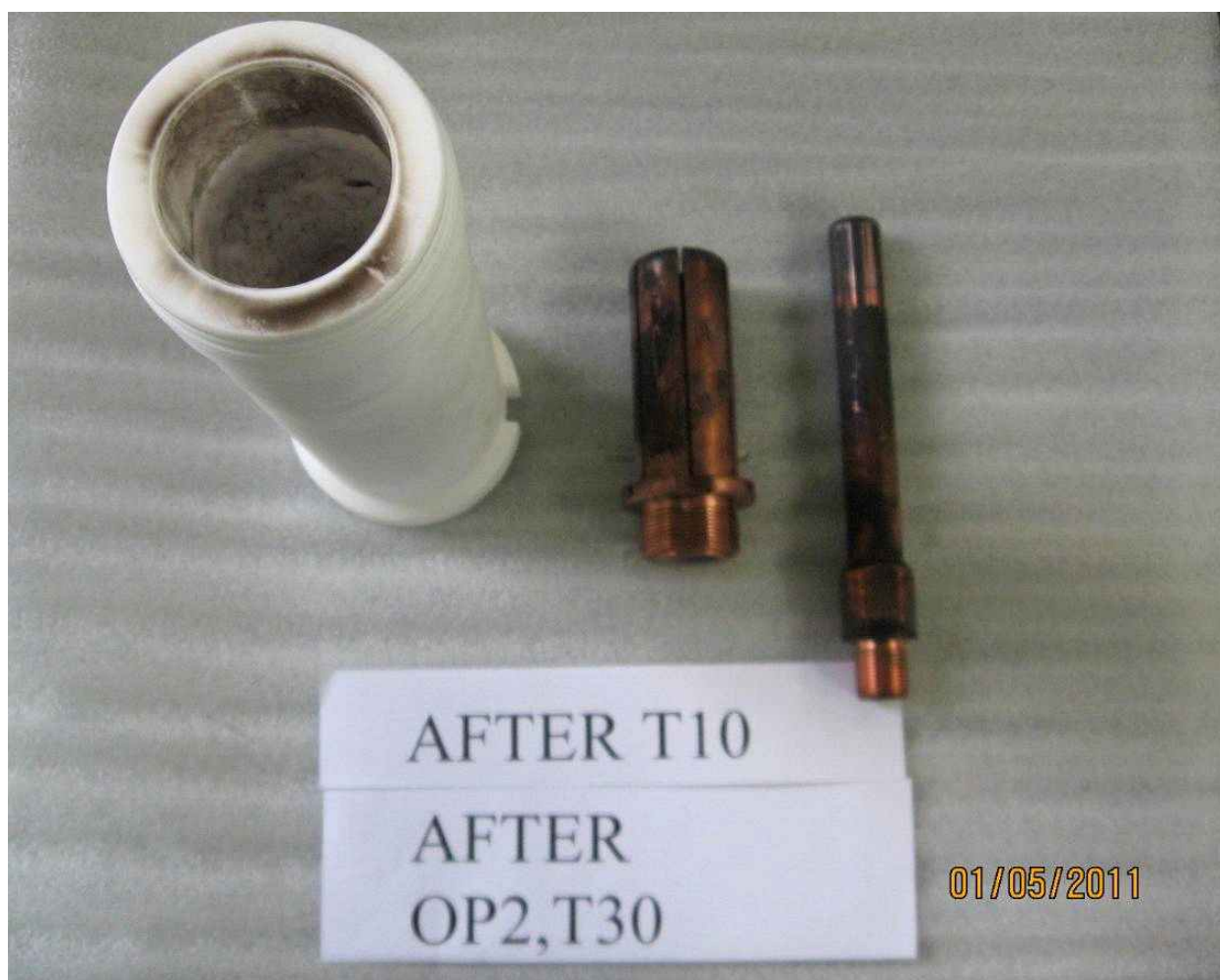
Photo. HP09 : Contact after basic short-circuit tests(T10, T30) and out of phase making and breaking(OP2)
