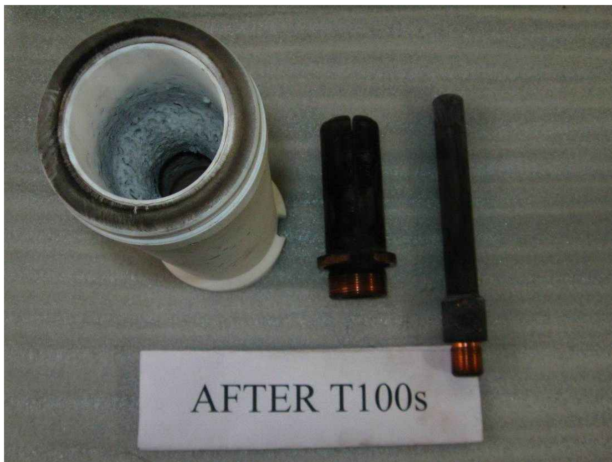
Photo. HP06 : Contact after basic short circuit test(T100s)
