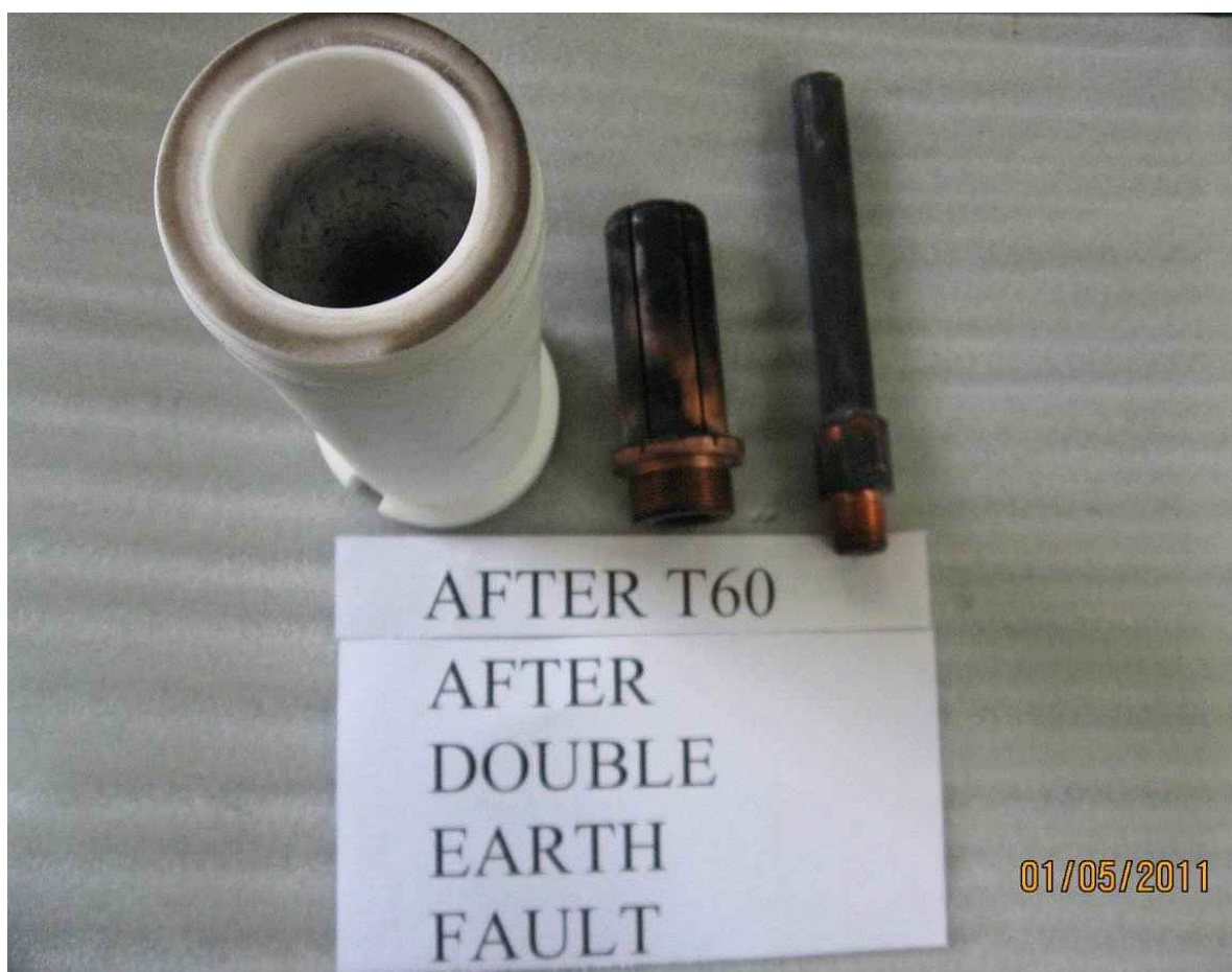
Photo. HP10 : Contact after basic short-circuit tests(T60) and double-earth fault test(DEF)
