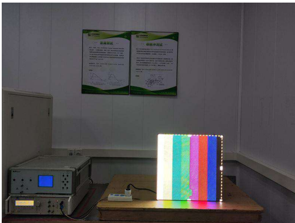
Photograph 9: Set-up for Harmonic & Flicker
