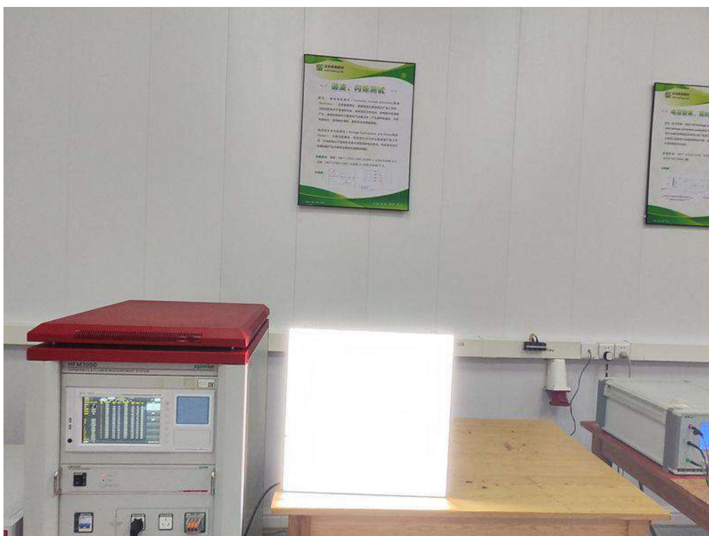
Photograph 9: Set-up for Harmonic & Flicker
