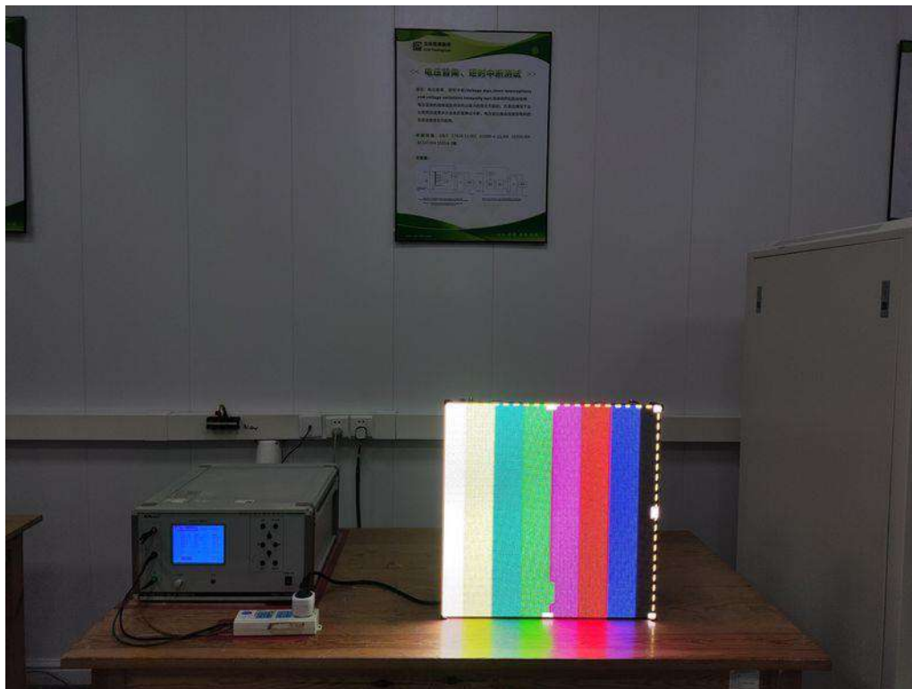
Photograph 7: Set-up for Electrostatic Discharges
