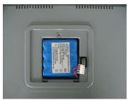
Figure 5-21 Battery installation
