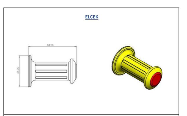
The material will be produced by injection molding technique from polyethylene material.
