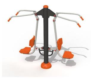
In the case of mobile elements, movement will be ensured by means of a joint system resistant to the external environment. The seats and backrests will be made of LLDPE polyethylene (linear low-density polyethylene) using "rotomoulding" technology. All mobile elements, heads, screws, nuts need to be covered with plastic protective caps.
