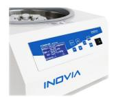
The FC5000 Series Desktop Centrifuges are provide a reliable and fast operation with the Brushless DC Motor and Micro Processor controlled system.
