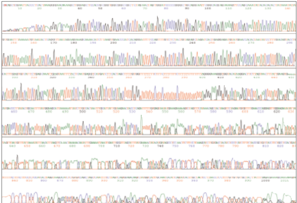
Figure 6. Longer Read Lengths with BigDye® Terminator v3.1 on the 3100 Genetic Analyzer. This figure shows accurate basecalling for more than 1,000 bases; the first ambiguity is not seen until base 1,040. The sample was run on the ABI PRISM® 3100 Genetic Analyzer with an 80 cm array using POP-4™ Polymer and the standard run module.
