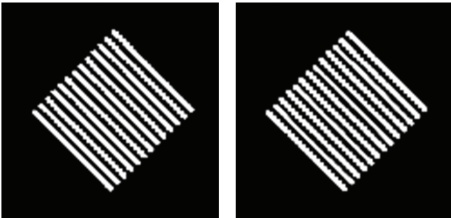
Figure 13: A single acquisition of a bar-resolution pattern of 8-line pairs/cm acquired using the ACR CT accreditation phantom (Gammex 464, Gammex). Images were reconstructed with FBP (left) and AIDR 3D iterative reconstruction (right). With the AIDR 3D reconstruction, spatial resolution is similar to FBP.
