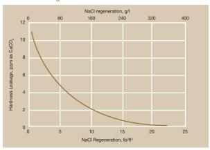
Capacity and Hardness Leakage graphs are shown assuming a service flow of 4 gpm/ft3 (32 l/h/l) and total dissolved solids of 400 ppm and 20 grains of total hardness. The hardness leakage will increase and the capacity will decrease while increasing total dissolved solids and total hardness.
