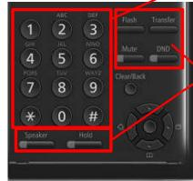
Six fixed feature keys for Handsfree, Hold, Trunk Flash, Transfer, Microphone mute & DND
