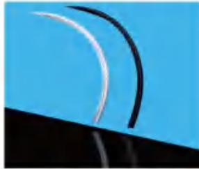
Comparison of black needle and ordinary needle under strong light
