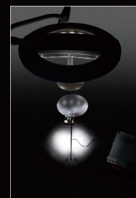
Shadow dilution with two masks 55%
