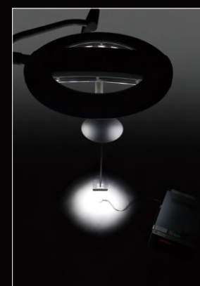
Shadow dilution with one mask 75%
