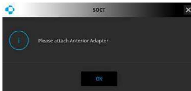
Once the adapter has been installed click **[OK]** to start calibration. To cancel the process and close the window click **[x]**. When Topography calibration is over the user is prompted to remove the Anterior Adapter and continue with WTW and Biometry calibration
