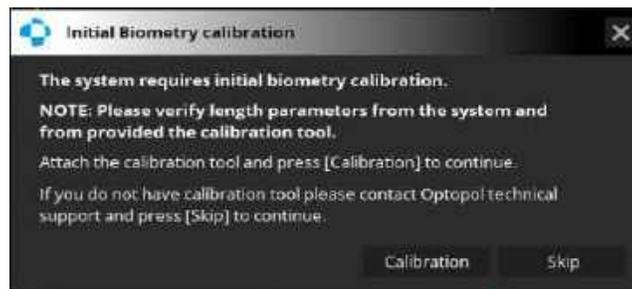
To skip calibration, click **[SKIP]**. The calibration prompt will be displayed on the next day. To start calibration, click **[CALIBRATION]**. If the calibration parameters provided with the REVO calibration tool have not been entered, the system prompts the user to do this, as shown below.
