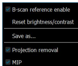
With the Maximum Intensity Projection (MIP) enabled the overlap of multiple vessels or projection (shadow) artifacts is ignored resulting in a cleaner angiogram as shown below.
