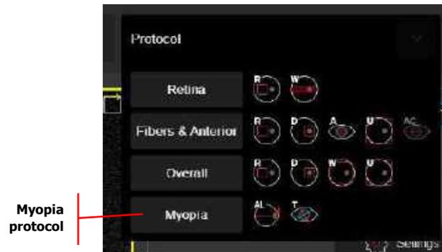
Before the start of the examinations software checks whether the calibration for biometry and topography has been done. If not, the SOCT will display a warning and ask to perform the calibration. When device is calibrated, the SOCT will start a biometry examination. After the biometry examination an acceptance window will appear. After accepting the biometry examination a topography examination will start. Also after the topography examination an acceptance window will appear.
