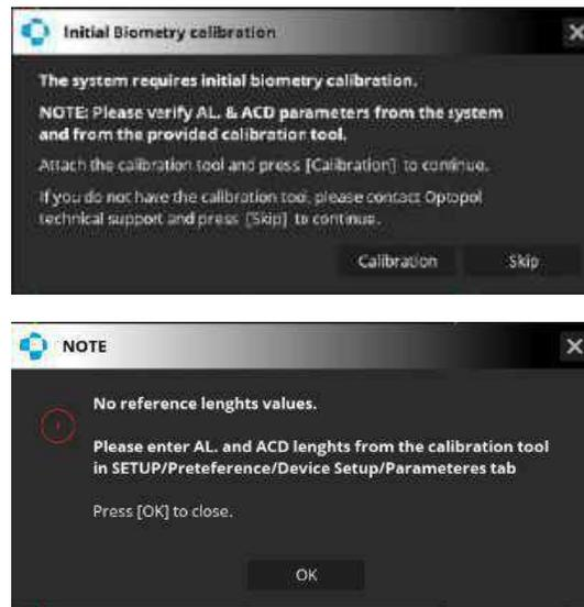
If the calibration parameters provided with the calibration tool have not been entered, the system prompts the user to do that, as shown below. Entering biometry calibration parameters is described in Chapter [22.1 Entering Biometry Calibration Parameters](#).
