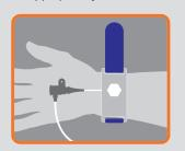
3. Insert band into slot on wrist plate Important: Ensure the device is applied firmly.
