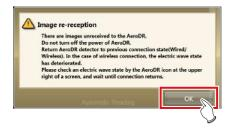
If there is an image on the DR Detector that has not been transferred when [ ] or [ ] is pressed on the exposure screen, a confirmation screen for reacquiring the images is displayed.
