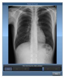
Only the image displayed in the current image screen appears in the serial exposure image output preview.
