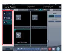
• If you press the exposure conditions display area where the reading sequence of the examinations is specified, the specified reading sequence is cancelled.
