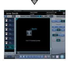
• Registration is performed in the patient database of this device, and the exposure screen or the body part selection screen is displayed.
