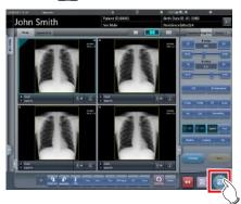
When the examination is finished, exposed images are batch output to a preset output destination.
