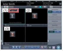
• Until the DR Detector is inserted into the wall stand and exposure becomes ready, "Preparing" is displayed in image display area (1).
