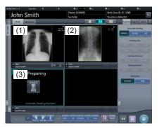
• When the DR Detector is removed from the wall stand, "Preparing" is displayed in image display area (3).
