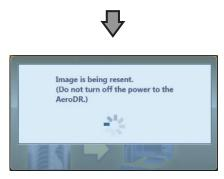
• When the connection is restored, images are automatically transferred.
