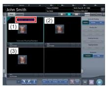
• In (1), "Panel not detected" is displayed until the DR Detector is inserted into the wall stand.
