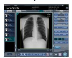
As soon as the exposed image is transferred, the image is displayed in the image display area.
