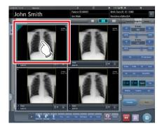
• The control panel automatically switches to the [Image Proc] tab. If it does not switch, select the [Image Proc] tab manually.
