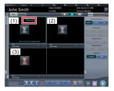
• When the DR Detector inserted into the wall stand is ready to start exposure, "Ready" is displayed.
