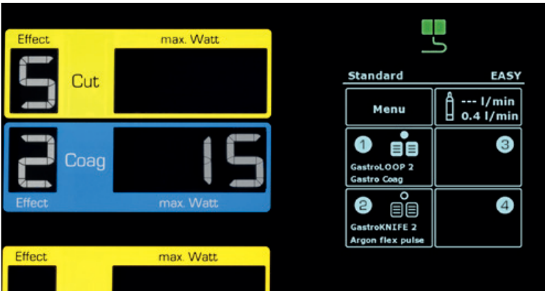
Highly flexible: GastroCut permits 6 cutting types with loops or knife electrodes for up to 9 effects
