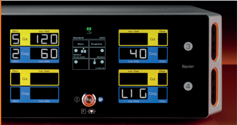
New: The LIGATION choice opens up new potential procedures and all settings are entered automatically
