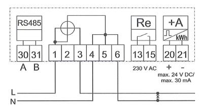
External tariff control, direct connection diagram, DIN terminal, unbalanced connection, SO output, RS485 interface.
