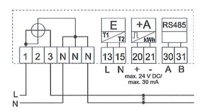
Internal tariff control, DIN terminal block, unbalanced connection, with supply control switch, two output relays R1 and R2 and RS485 interface
