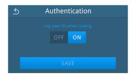
3. After a setting has been changed, the SAVE button is active. Press SAVE to accept the setting.
