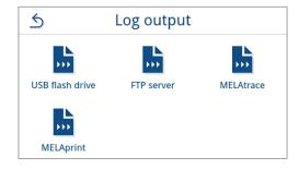
3. Press on or off to activate or deactivate the immediate output.
