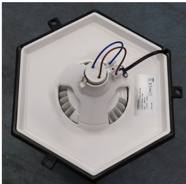
Photograph No. 48 Components plate after removing the cover.
