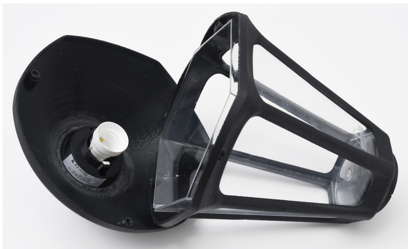
Photograph No. 29 Luminaire after removed the cover
