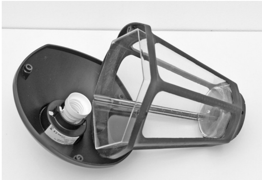
Photograph No. 12 Internal cover, with lampholder
