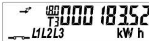
Figure 6. Active energy (A +) in total by phases and rates
