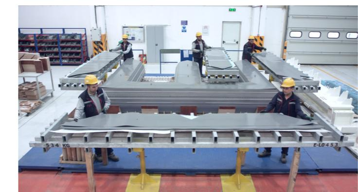
The cores of the transformers are made of silica sheets with oriented cores produced by cold rolling.
