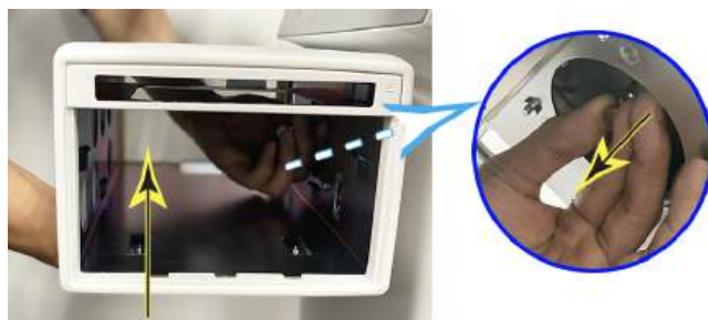
Figure 3-103. Pull out the locking pin
