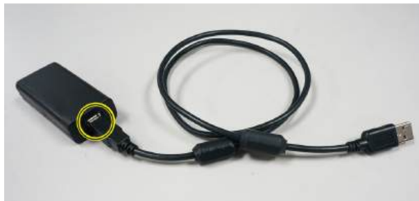
Figure 3-45. Insert the USB connector into Printer USB Isolator
