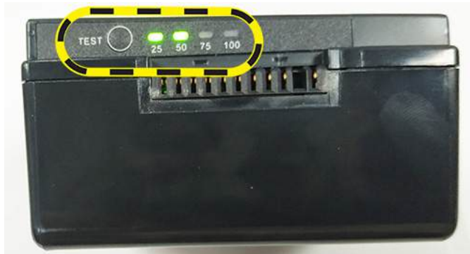
Figure 7-43. Press TEST Button
