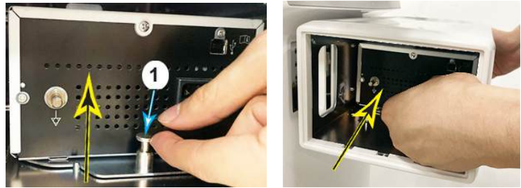
Figure 3-104. Lift the locking pin
