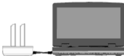
Figure 3-51. Discharging: 2pcs spare battery + console battery
