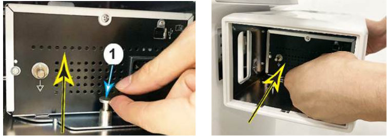
Figure 3-101. Lift the locking pin
