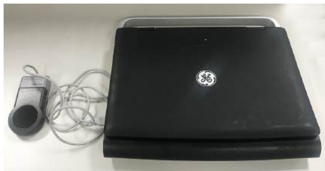
Figure 3-33. Connect Footswitch to the system (2)
