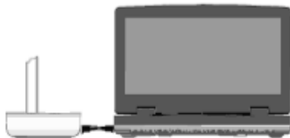
Figure 3-50. Discharging: 1pc spare battery + console battery
