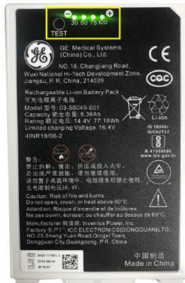
Figure 7-42. Press TEST Button
