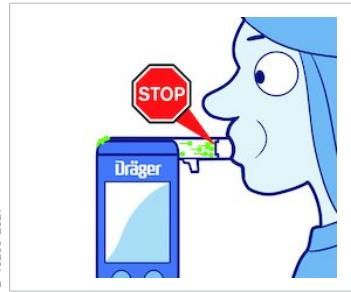
With a non-return valve, the intake of potentially contaminated air is not possible.
