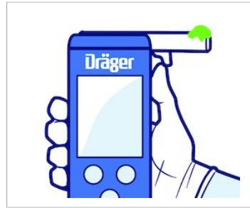
The spacer prevents direct contact of the lips with the instrument.
