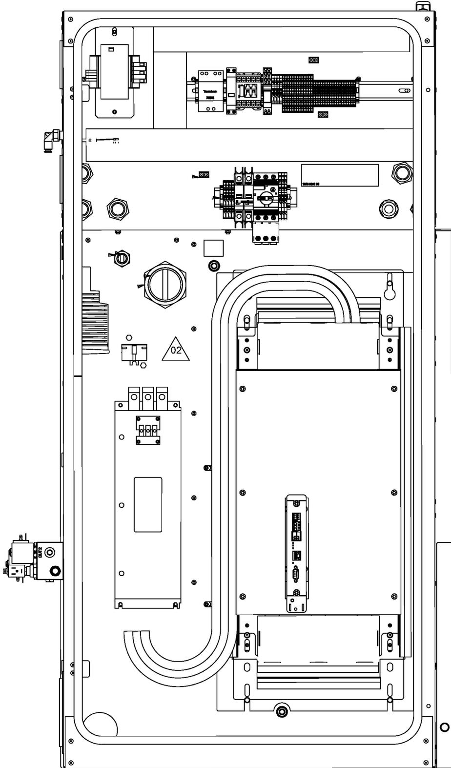
**19.11 - Cubicle components GA 45 VSD+ - 200V-400V-500V/50Hz,
