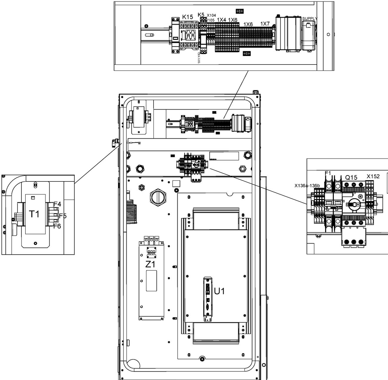
**19.9 - Cubicle components GA 45 VSD+ - 200V-400V-500V/50Hz,
