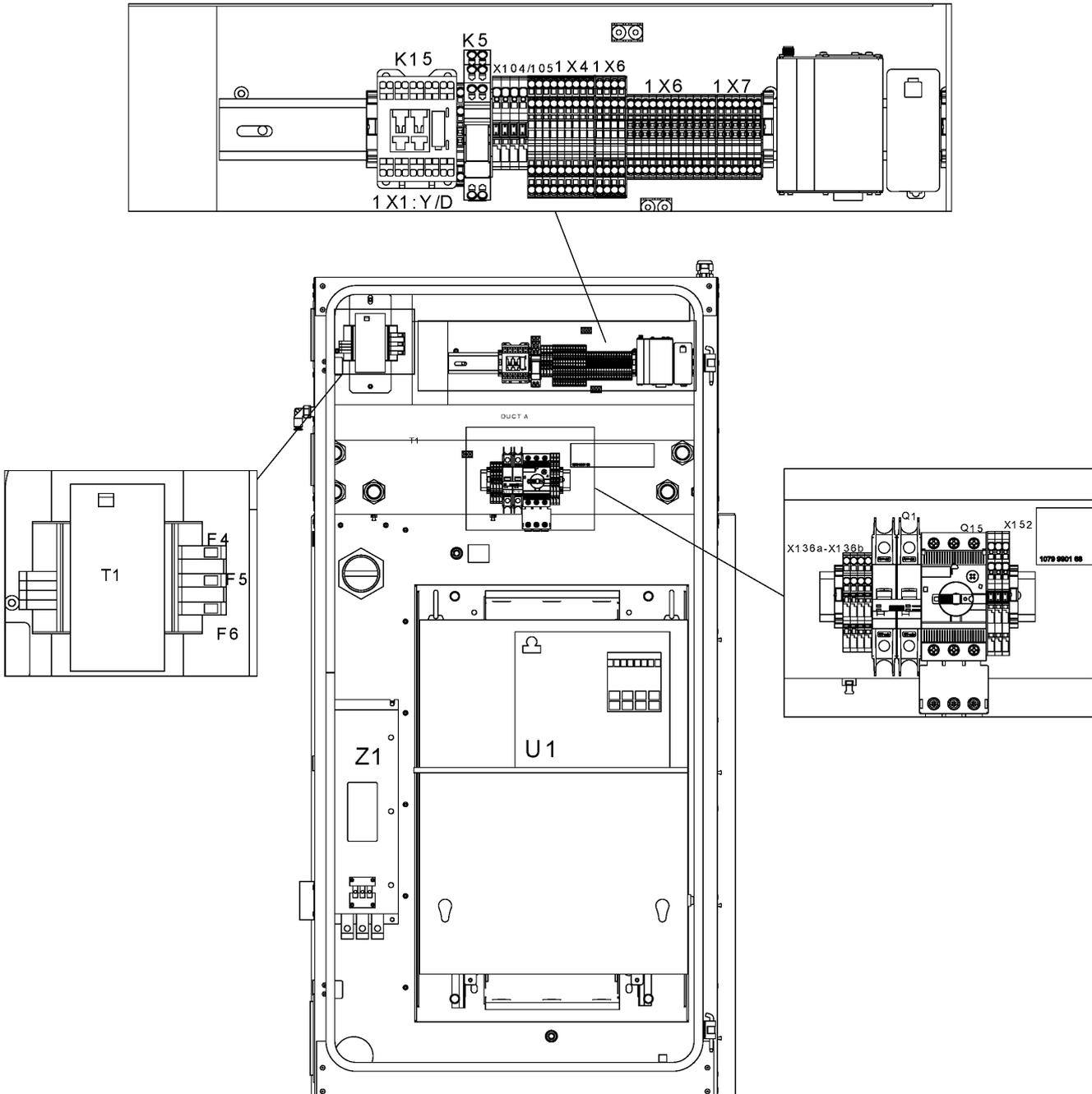
**19.3 - Cubicle components GA 37L VSD+, GA 45 VSD+ - 460V/60HZ (06/05/2016 - 14/11/2017)**
