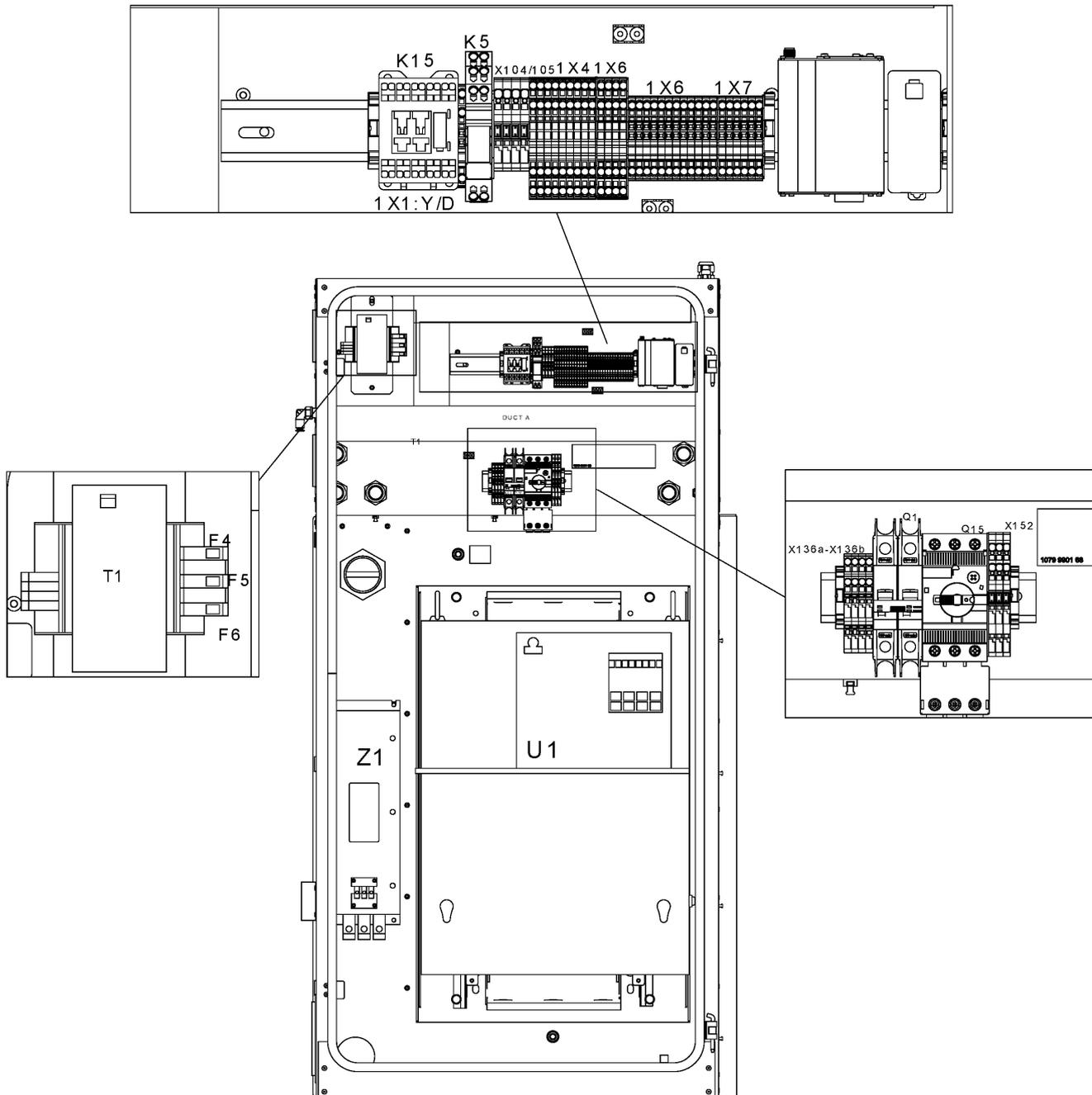
**19.8 - Cubicle components GA 45 VSD+ - 200V-400V-500V/50Hz,
