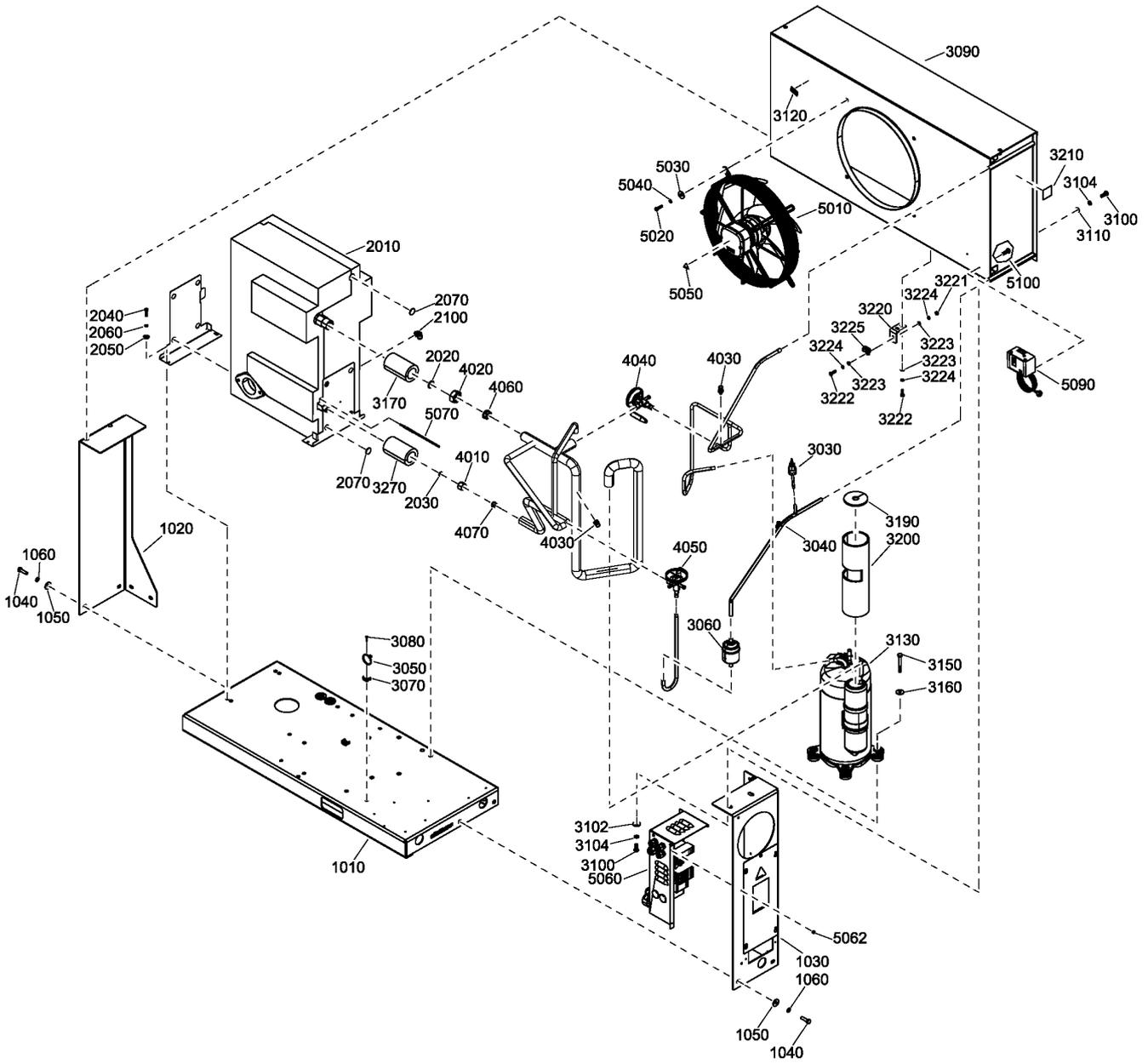
**18.3 - Components GA 37L VSD+, GA 45 VSD+, GA 55 VSD+ - ID180 - 460V/60Hz IEC, 230V-460V/60Hz UL-cUL**
