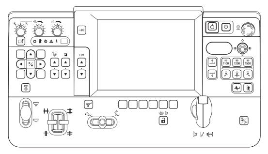
Some of the buttons and levers on the console are connected with the movement of the X-ray diagnostic table and some are connected with X-ray irradiation. They are explained according to function.
