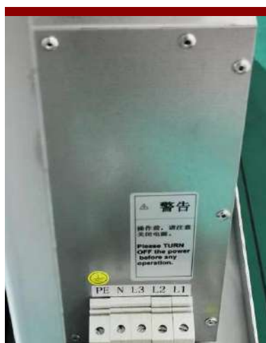
Figure 2-2 Three phase-five-wire connection
