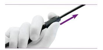
Press movable ring part of the handle forwards and hold at this position. Pull back spring mechanism of the axial handle as far as it will go and hold it. Take the shaft at the distal tip, push shaft into the spring mechanism as far as it will go and join with a slightly rotary movement.
