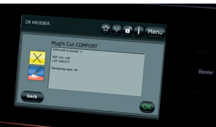
Plug'n Cut COMFORT: The COMFORT SYSTEM automatically recognises the COMFORT instrument, indicates how many times it may still be used and selects the correct parameters for the procedure
