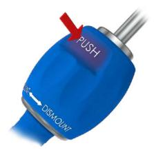
Tips 1 and 2 of wrenches for screws are exchangeable. In order to disconnect the tip from the wrench [40.8090] or [40.8089], press and hold the PUSH and then remove the tip from the wrench sleeve.
