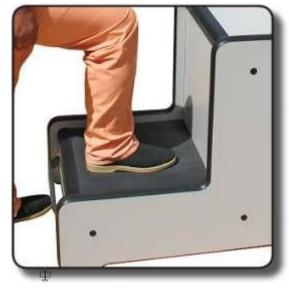
Note: if the operator is scanning one(1) foot at a time, the best foot position is with the foot centered front to back and with the center of the foot position two (2) inches off center right or left on detection zone.
