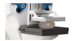
Once in contact with breast the compressor briefly stops and starts to increase compression force. Basing on breast density the microprocessor controlled system evaluates if reaching the selected force value or if stopping the compression at 100 N.
