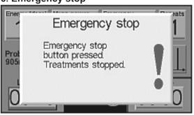
stops power supply of applicators. Turn the device off and on again for further use.
