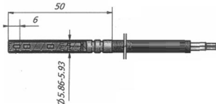
Fig. B3.2 Overall dimensions of the PL type temperature sensor
