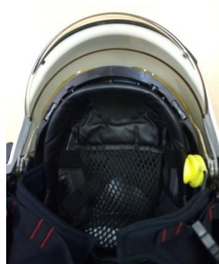
Fig. 8 Attaching plate with fixed communication system. Communication system holder. Loudspeaker.
