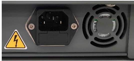
Figure 14 – Replacement of the fuses: fuses box
