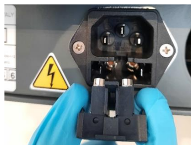
Figure 17 – Replacement of the fuses: repositioning box
