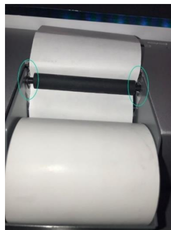
Figure 18 – Printer paper replacement: roll off axis
