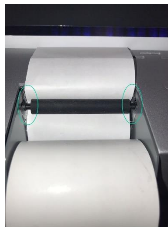
Figure 20 – Printer paper replacement: correct position
