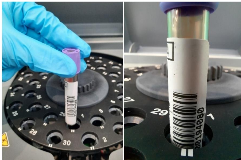
Figure 24 Correct insertion of the test tube
