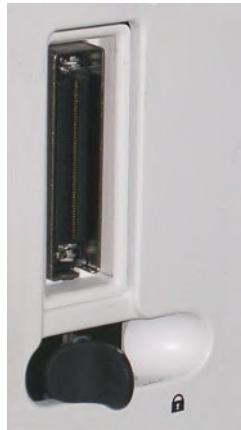
Figure 3-18. RS Probe Connection Locking Lever
