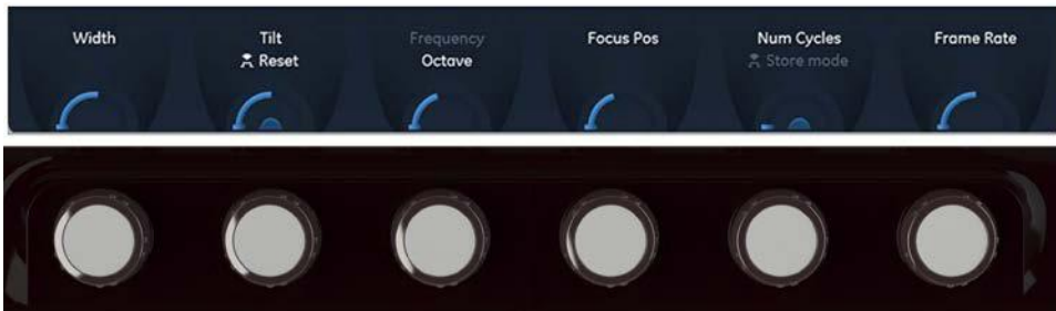
Figure 3-29. The Rotary/Push buttons
