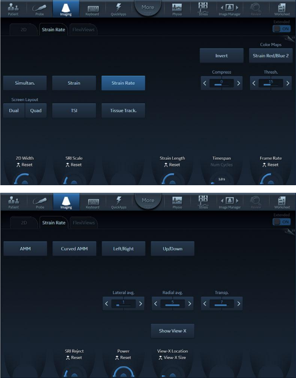
Figure 5-16. The Strain rate Touch Panel page 1 and 2
