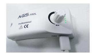
Plug the charging cable into the POWER port. It is charging when the indicator light is flashing. When all 4 indicator lights are on and not flashing, the battery is fully charged.
