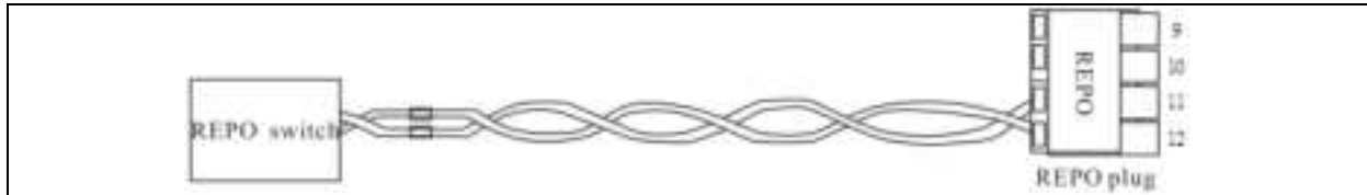
Figure 7.3 REPO Cable Connection
