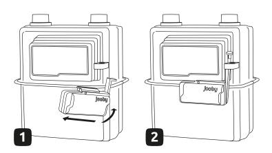
Make sure that the LED indicator flashed once at the moment of installation. You should also see six short flashes within 1 minute. This means that a radio exchange took place between the radio module and the service provider gateway.
