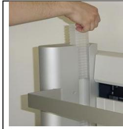
1. Remove a strip of cuvettes from the package.
