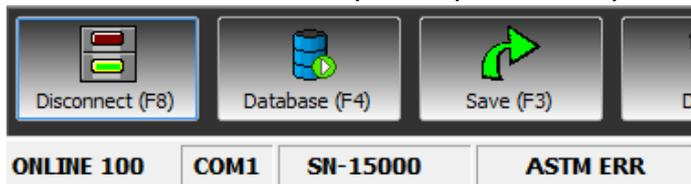
TECAM is linked to system "15000" over com port 1. No ASTM is active
