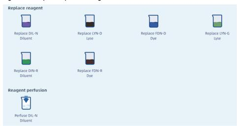
If the main unit disables the RET channel, the reagent replacement interface only displays the icons of diluent and lyse. If you need to disable the RET channel, contact Dymind customer service department or the local agent.
