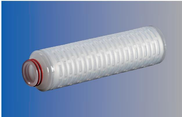
BGH Series filter cartridges are comprised of multi layers of media. This filter structure provides excellent flow rate at low pressure drop and high throughput, while achieving submicron retentions, high efficiency, and extraordinary dirt holding capacity. The filter media and its support structure are thermally welded to the end caps, ensuring minimum extractables of integral filter cartridges in a wide range of applications.
